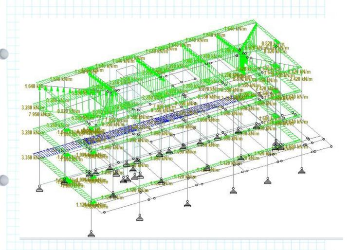
Wind load on members for the case of Wind - Z (CPE + CPI) Direction
