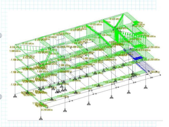
Wind load on members for the case of Wind - X (CPE + CPI) Direction
