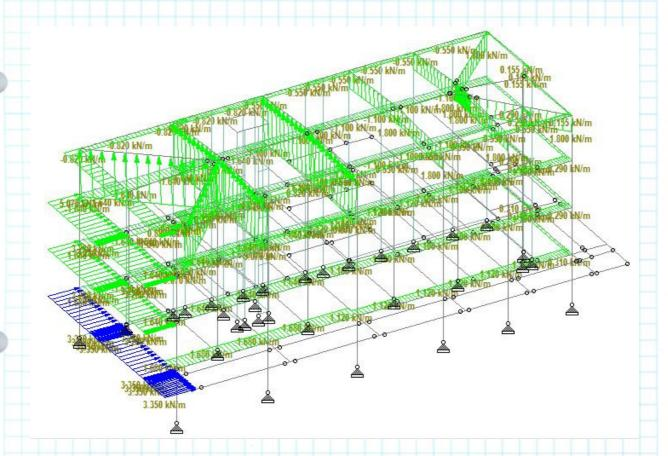
Wind load on members for the case of Wind + X (CPE + CPI) Direction
