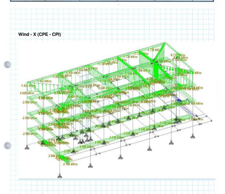
Wind load on members for the case of Wind - X (CPE - CPI) Direction
