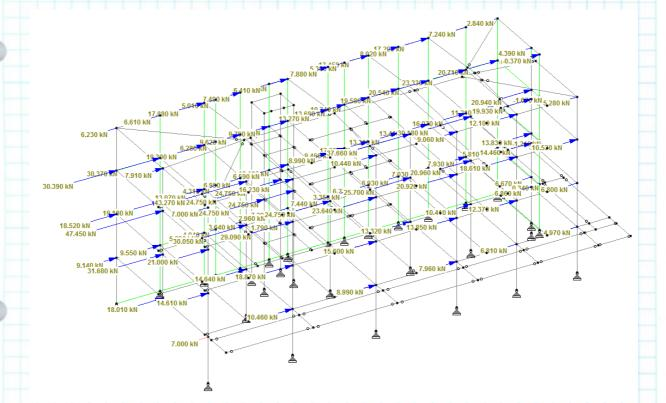
Earthquake load on joints for the case of Earthquake +X Direction
