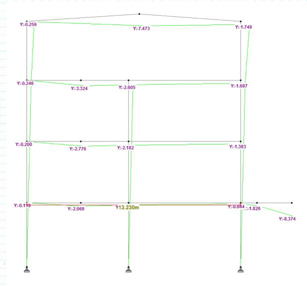
Load 201: Displacement Displacement - mm
