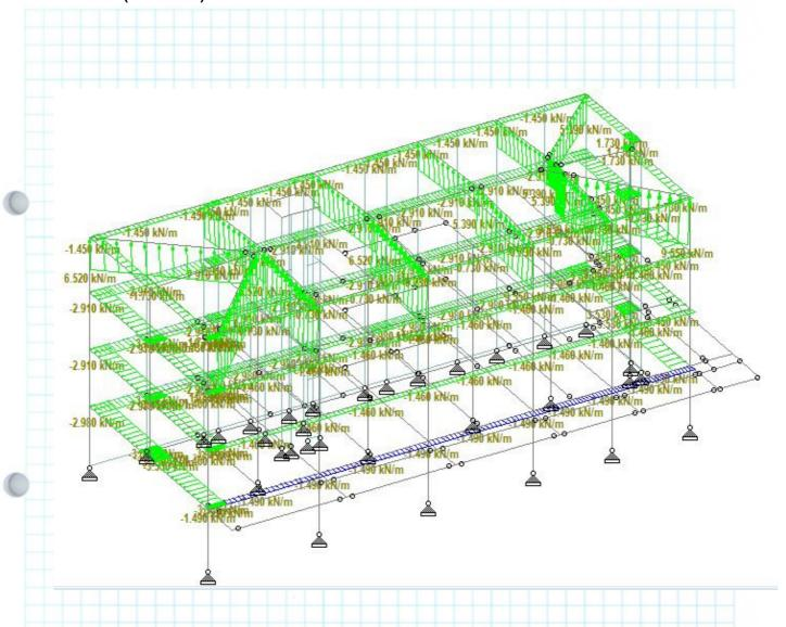
Wind load on members for the case of Wind + Z (CPE - CPI) Direction
