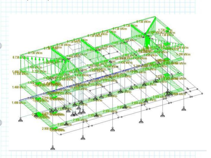
Wind load on members for the case of Wind - Z (CPE - CPI) Direction
