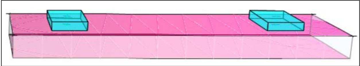
SAFE modeling of CF8 foundation as finite elements
