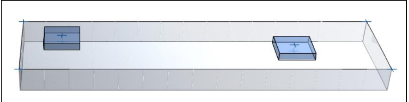
SAFE modeling of CF5 foundation as finite elements
